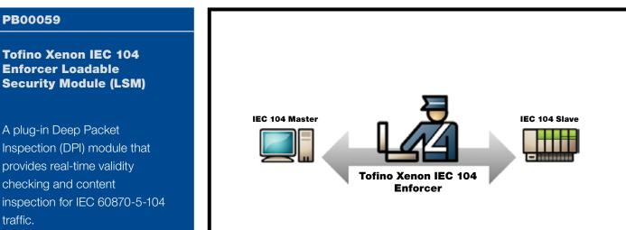
The Tofino Xenon IEC 104 **Enforcer LSM makes sure that** the only IEC 104 commands your control devices receive are approved commands from approved computers.
